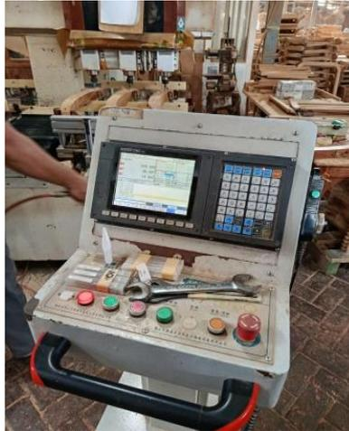
Gambar 2 – Unit Kontrol Mesin CNC
